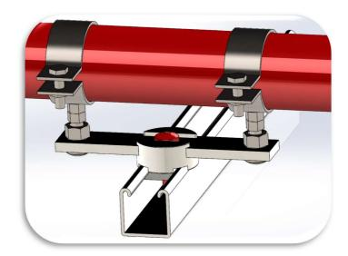
This is an Anchor Point, designed to rigidly fix pipework. The LWFA is perfectly designed to clamp onto 41mm Strut Profiles. Recommended profile is 41x41x2.5mm
